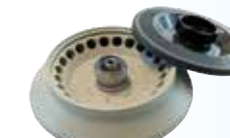
Angle rotor, 24-place, Cat. No. 01226 n = 13,300 min -1 , max RCF 17,008
